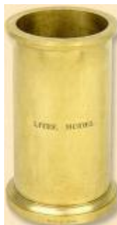
Figure 2. Litre Standard in brass (1802)
